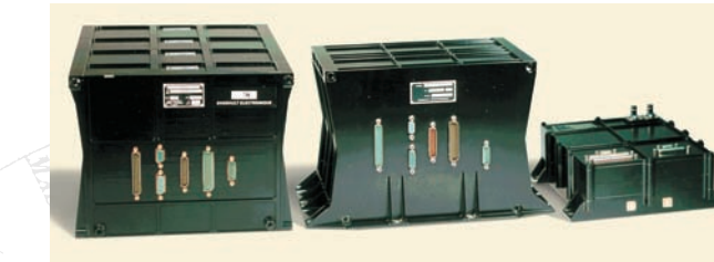
First (SPOT-2, SPOT-4, TOPEX/Poseidon), second (Envisat) and miniaturized second (Jason, SPOT-5) generation on-board DORIS receivers CNES
