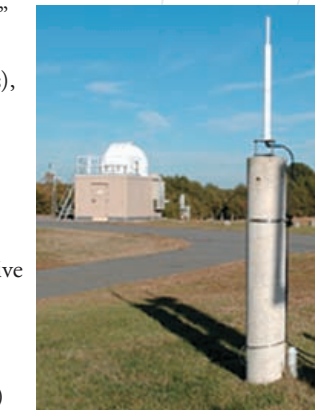
DORIS antenna at NASA GSFC (SLR2000 in background)
